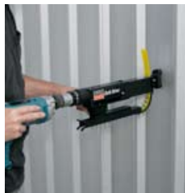
Individual profile guides fit flat profile of cladding sheets, corrugated-profile metal roofing sheets, and ribbed/square profile of square-ridge metal roofing sheets.
